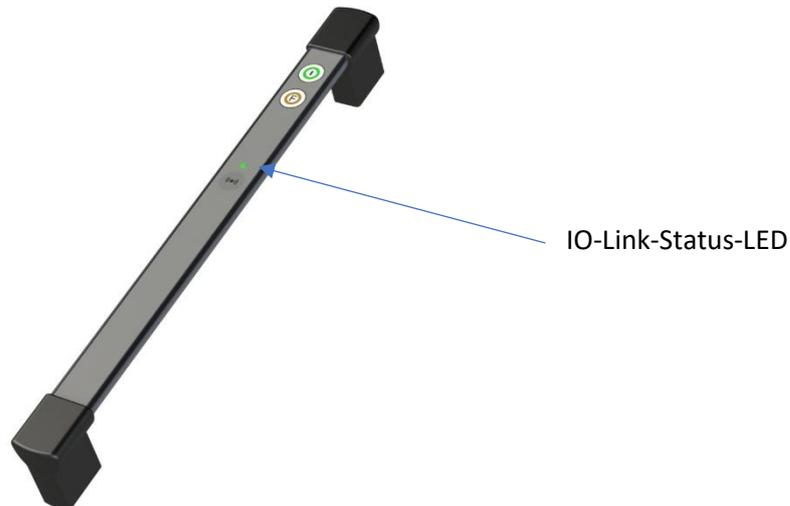
A status LED is clearly visible on the signalling device. In normal operation, this status LED indicates the IO-LINK status in GREEN. If device errors are detected with the integrated self-diagnosis, the IO-LINK status changes to the colour RED.
